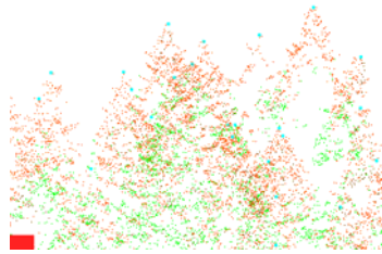
(b) Raw LiDAR points with consensus sets and maximum points.
